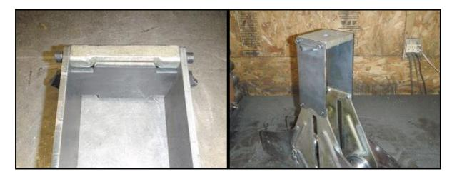
**Step 4.** The pin below is attached to the pipe clamping vise that comes in the electric pipe threading kit from Harbor Freight. You will need to press out this pin out of the clamping vise. The total length needs to be  $\sim$ 5" long. If pressing the pin out is difficult you may also cut it out of the vise.
