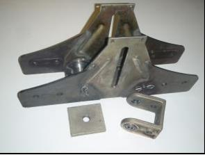
**Step 3.** Install the parts as shown below, using the provided 5/16" fasteners on the bottom. If you have an earlier model tubing bender you will need to enlarge the rectangular window down 3/16" in order to insert the spring mount.
