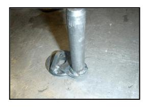
**Step 6.** Install the 20MM pin and bottom spring mount bracket as show below in the first picture. Be sure to keep the cotter pin parallel to the ground, as the opposing side of the pin will get the anti rotation bracket welded to the shaft, first tack into position and make sure the top die assembly freely slides up and down then fully plug weld the 20MM pin to the anti rotation bracket.
