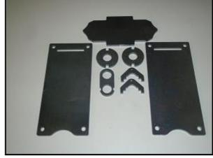
**Step 2.** Dismantle the HF tubing roller down to the three pieces shown below.
