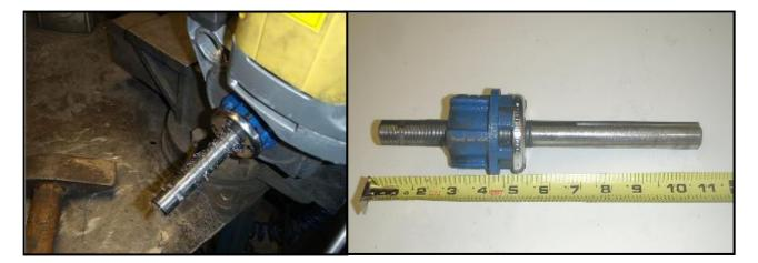
**Step 8.** Install the drive axle, 4 ton bottle jack clamp, and springs as shown below.
