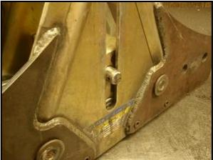
**Step 7.** Using the ½" pipe thread die that came with the HF pipe threader, remove the 4 Phillips screws and remove the chrome cap off the ½" pipe die, take a punch and pry back the 4 cutting teeth. This will allow you to slide the die ~2.75" down on the shaft then tack weld the die into position as shown below. Be sure to center up the die prior to welding, this will reduce the wobble of the pipe threader when installed.
