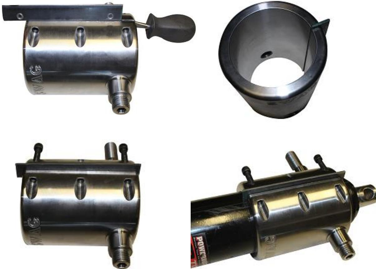
Remove the two 2" long bolts when the clamp assembly is positioned as close to the edge of the ram as possible just before the rolled edge of the cylinder and the short threaded stud is pointed in line with the machine thumb knob installed in step #2.
