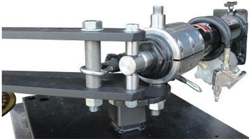
The pictures below are of the JD2 model 32 tube bender which uses the 1<sup>st</sup> and 3<sup>rd</sup> hole locations to mount your tube bender to the mounting pedestal, as illustrated below. If you own a different model of tube bender you will use the 1<sup>st</sup> and 2<sup>nd</sup> mounting holes
