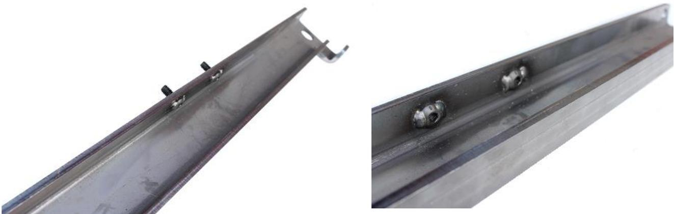
Square up and center the bottom die to the press brake frame using the top die to help center the bottom die. Tack all four corners of the die first to reduce warping of the press brake frame. Next, fully weld the bottom die into position alternating sides while welding a few inches at a time. (If necessary, grind the bottom edge of the angle iron so it sits flush against the bottom formed channel)
