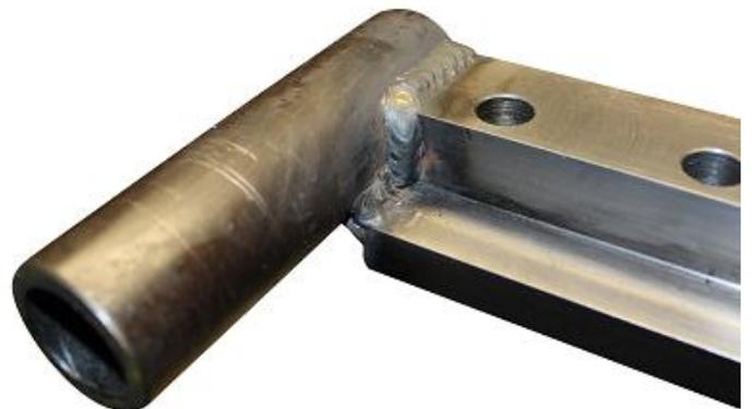
Depending upon the thickness of your weld it may be necessary to bevel the edge of the 1/2" thick threaded beam clamp to ensure it sits flush as shown below.
