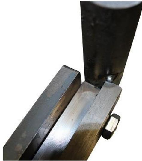
Next, tack the guide tube in a couple different locations. (double check that the top die assembly will freely slide on the vertical guide rods welded in Step 1.) Adjust as necessary. Next fully weld both sides of the guide tubes to the machined side of the clamp assembly. (REMEMBER: Take time to protect the machined area where the finger dies are clamped. Welding spatter will easily stick to the clean machined surface if left exposed and prevent proper clamping of the finger.)
