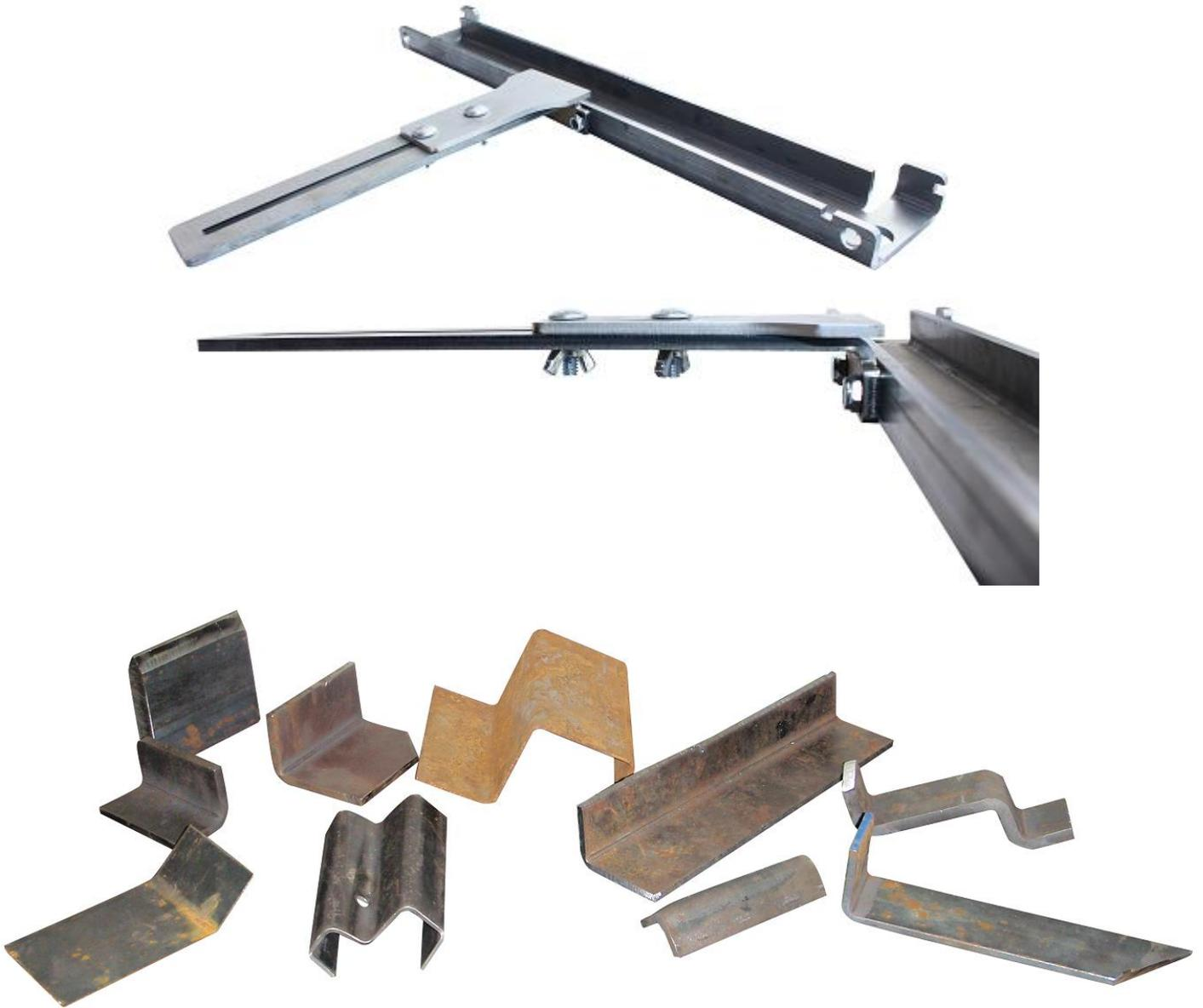
**IMPORTANT NOTES:** It is critical that you support the entire bottom side of the press brake. Failure to do so will destroy the press brake! (ask us how we know)
