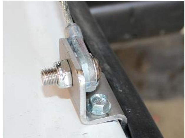
Install the 3/8"x 1" SS bolt, 3/8" nyloc nut and 3/8" washers. When tightening the 3/8" bolt, the cable eyelet should be just loose enough so it can freely pivot around the bolt without rattling.
