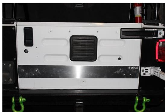
Align and install the aluminum panel using the two mounting holes on the passenger side of the tailgate. Using the aluminum panel as a template, mark the 6 holes to be drilled in your tailgate, shown by the red arrows below.
