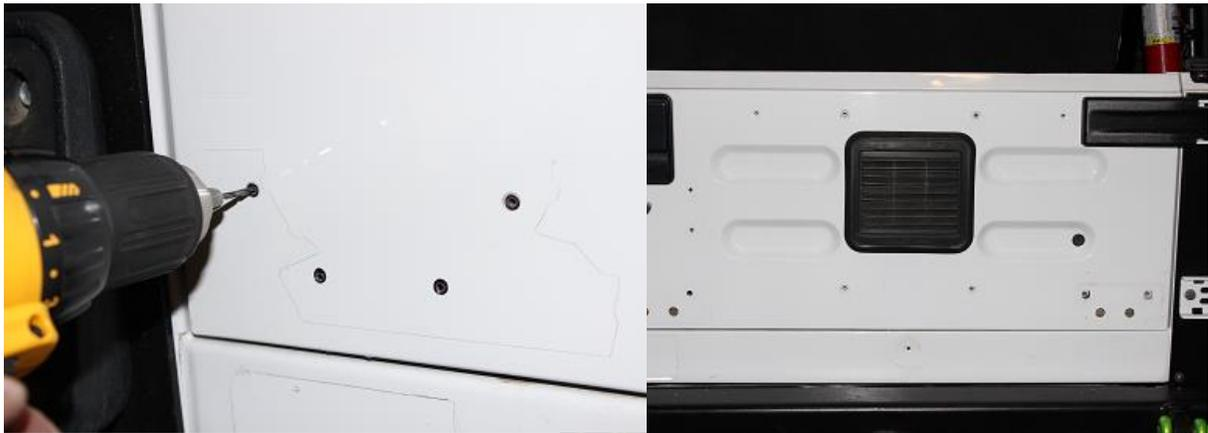
Enlarge the two 21/64" holes on the inside of your tailgate to 1/2" diameter. This will allow you to pass a 1/2" deep wall socket into the hole and tighten the aluminum panel to the tailgate.
