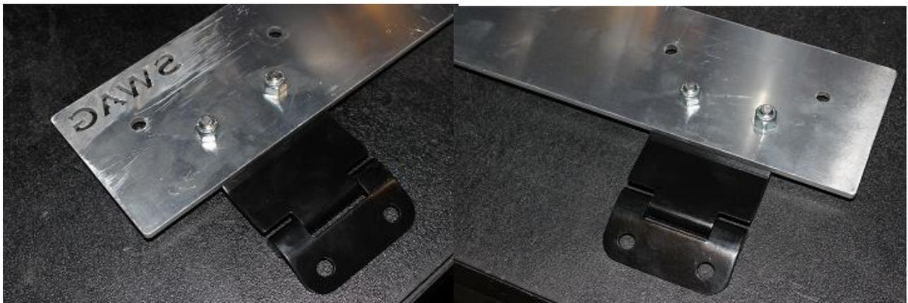
Install the aluminum panel on the tailgate using the provided 5/16" SS fasteners on the passenger side. On the driver side install the 5/16" ss fasteners, and on the backside install the 5/16" washers and nuts. Tighten the nuts with a 1/4" deep wall socket.
