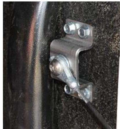
The tailgate cable tub brackets are attached with (4) ¼” self-tapping screws. When tightening the 3/8”x1” SS bolt, nyloc nut and (1) 3/8” washers the cable eyelet should be just loose enough so it can freely pivot around the bolt with our rattling.
