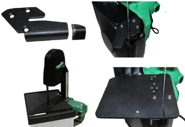
then install the portaband table using the same two Phillip's head screws that came with your saw.
